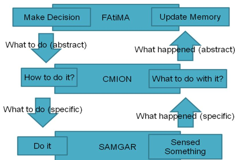
The next diagram explains in more technical detail how the architecture components are connected:
