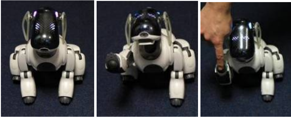
Figure 21. AIBO expressing Boredom behaviour (attention seeking) - in this behaviour AIBO executes a combination of movements, sounds and LED display in order to attracts the user's attention. It then lifts its paw and waits for the user to interact with it (pressing its paw).
